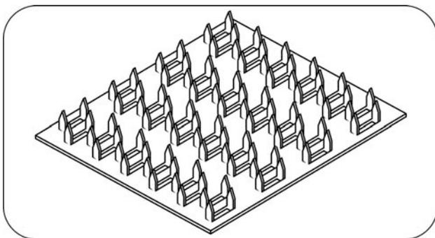
**Figure 1.** Drawing of a typical truss plate.
