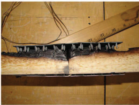
Figure 14 - Post burn - 1/32 in. wood/plate gap specimen
