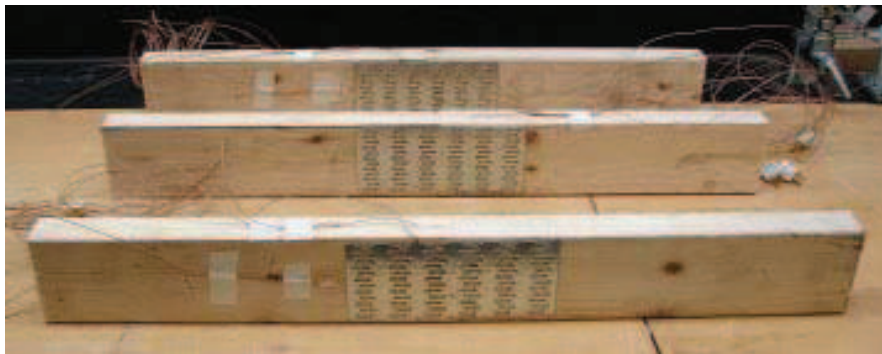
Figure 2 – Typical set up of test members
